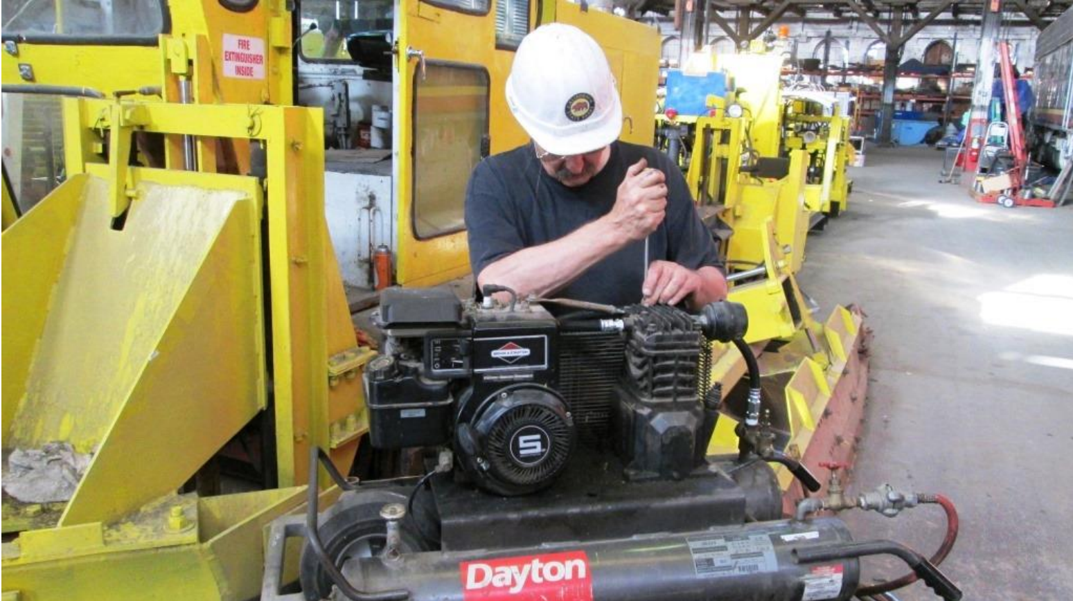
Fred makes the permanent repair to the air-compressor on a cart
