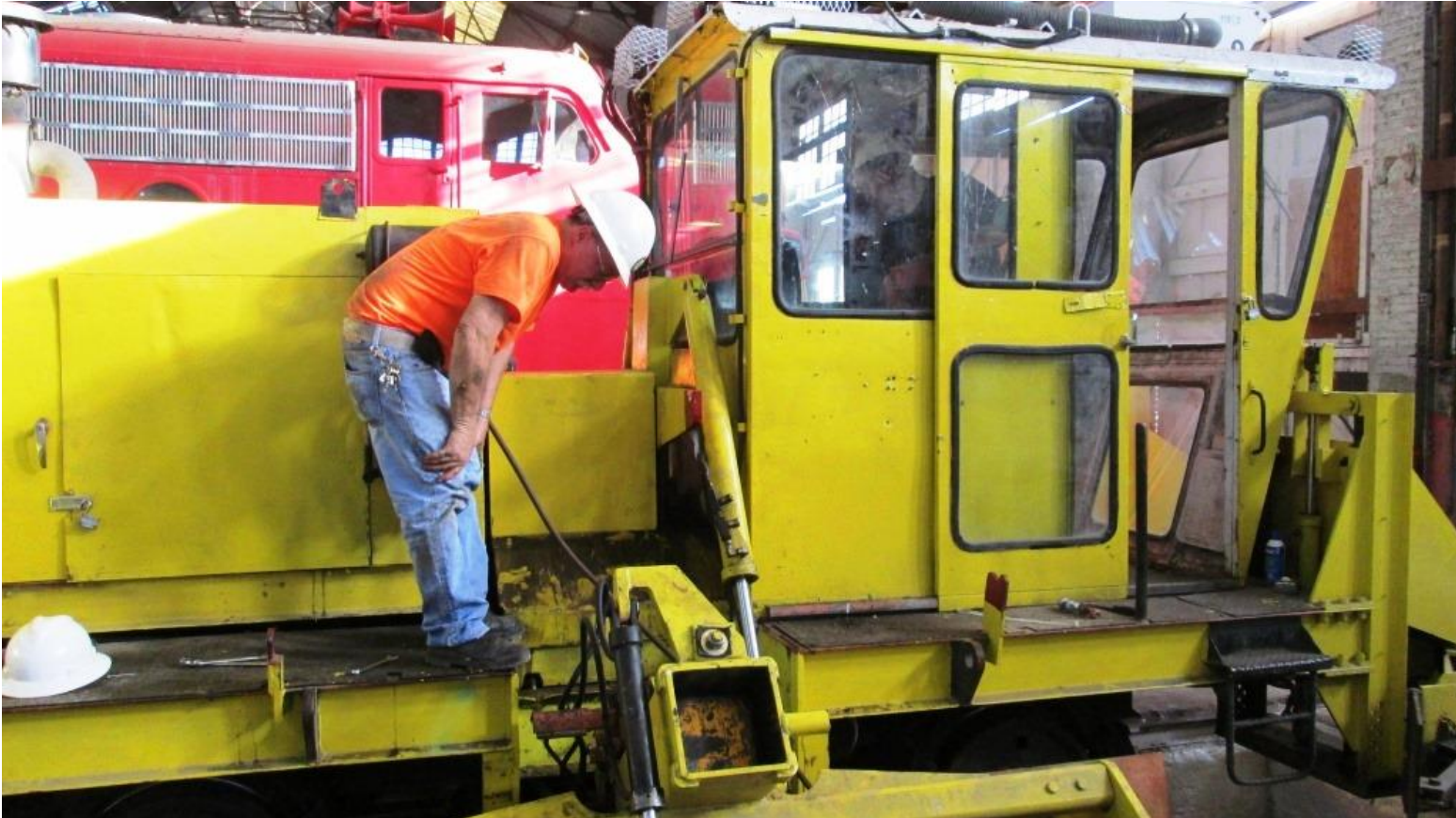
Mike H. and Fred (in the cab) adjust air-actuated systems on the ballast regulator
